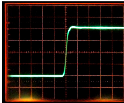
Transition time is 7 ns and overshoot is less than 2% (20 ns/div)
