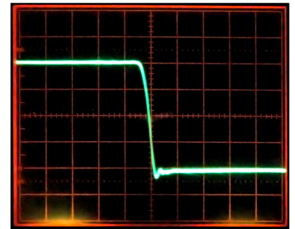
Transition time is 9 ns and undershoot is minimal
