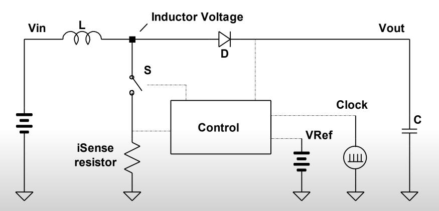
When the balance point is reached, Switch S opens, and inductive energy is transferred to the output.
