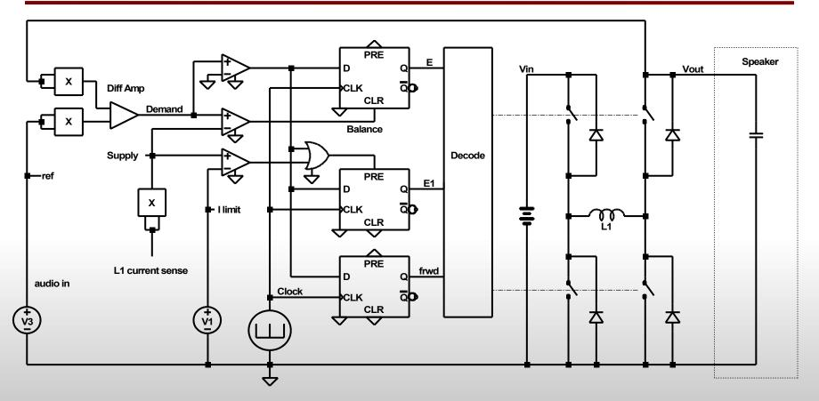
Audio amplifier to drive a cell phone piezo (or dynamic) speaker more efficiently from a 4 volt battery.
