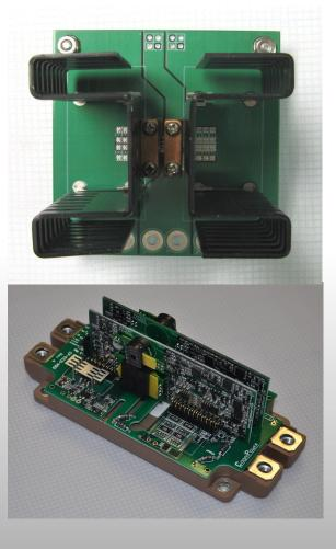
CogniPower is developing an AC-DC topology that performs Power Factor Correction and agile output regulation in which the majority of power moves through only a single stage of power conversion. Better efficiency and smaller size result.
