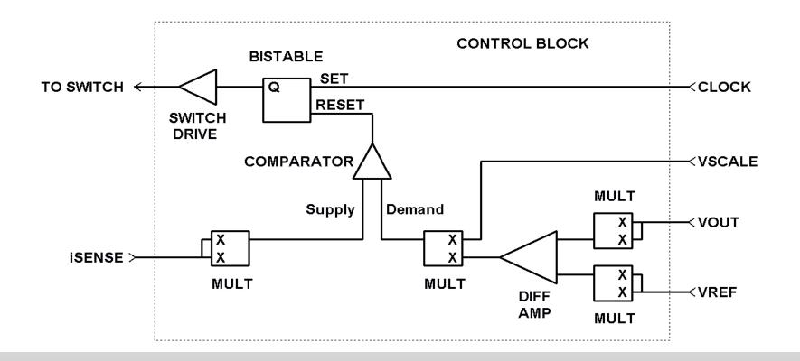
A generalized circuit block can perform the Energy Balancing calculation for a variety of SMPCs.
