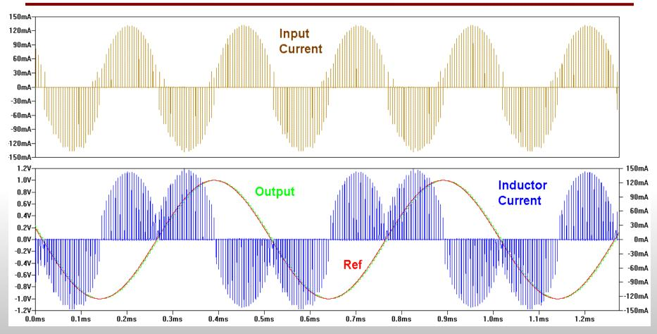
A bipolar output is generated from a unipolar input.
